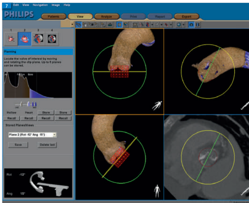
▲ Figure 7. Planning the procedure. The green circle represents the view from the X-ray system and the yellow circle is perpendicular to the green circle. The view can be changed using the Rotation Interactor. The C-arm orientation indicator shows the system angulations corresponding to the top-left view. In the 3D volume rendering of the CT aortic root, calcifications are automatically shown in blue. The red mesh indicates the planned device.
